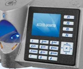
IP 65 rated for operating in Severe Downpours, Ice and Snow
